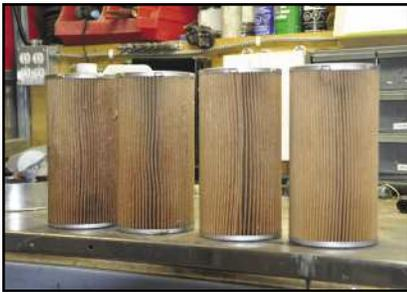
Each of these filters appears to be similar however, they vary according to their weight. Filter 1 (far left) is clogged with biofilm and was inhibiting the operation of a boiler fuel system operating on ULSD. Fuel Right was introduced into the fuel storage tank with each delivery of fresh fuel. Over a four month period, the filters progressively improved. Filter 4 remains a fully functioning filter with the biofilm presence eliminated with no filter clogging evident.
