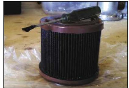
fouled marine filter from a Racor water separator
