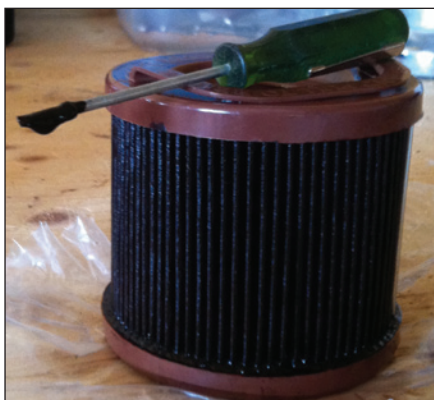
Image 3: A marine filter/water separator plugged with bio-film. Treatment of the fuel with Fuel Right® dissolved the existing sludge in the fuel tank.
