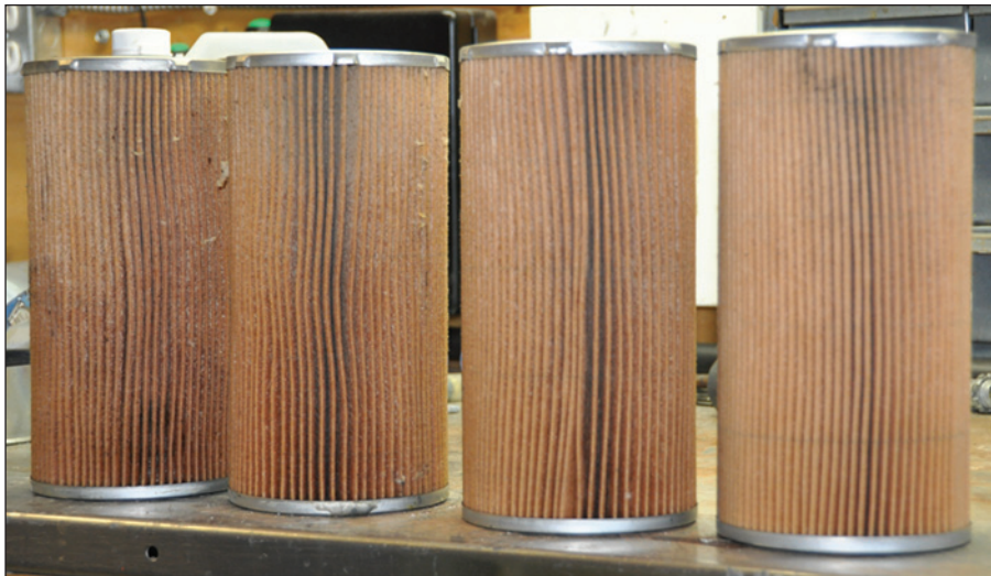
Image 2: Filters from a boiler system operating on ULSD. Fuel Right® filming amine technology was used to treat the fuel and over a three-month period, the bio-film (opaque) was dissolved and filter plugging issues were eliminated. The fuel was sloughing deposits of bio-mass downstream and prematurely clogging filters. The bio-film is opaque. The weight of the filters reduced from left to right due to reduction of bio-film loss.
